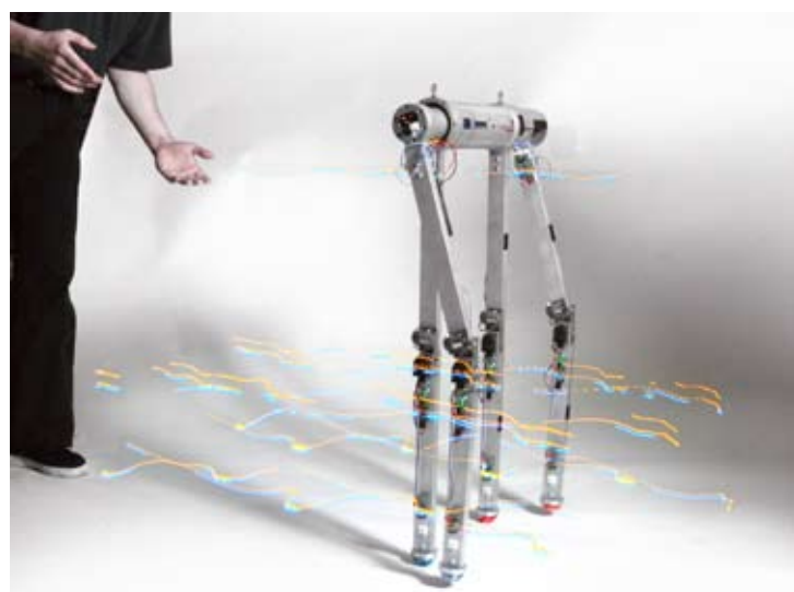
Dribble was made by the group of Stefano Stramigioli at University of Twente, in Holland. It is a 4-leg "biped".
